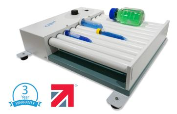
Heavy duty Clifton Roller Mixer for vials, small bottles, and test tubes. Durable design for mixing solid and liquid suspensions and viscous liquids, featuring rugged sprocket and chain drive, coupled with ball race roller mountings for smooth trouble free operation and can run continuously for many hours unattended using powerful DC motor.
